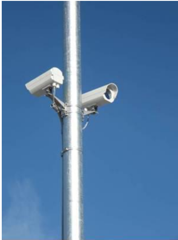
Figure 92. An area-cover animal detection system (passive infrared, manufactured by ADPRO (Xtralis, USA)), designed to detect large mammals on both sides of the pole, at a WTI-MSU test facility near Lewistown, MT (copyright: Marcel Huijser).
