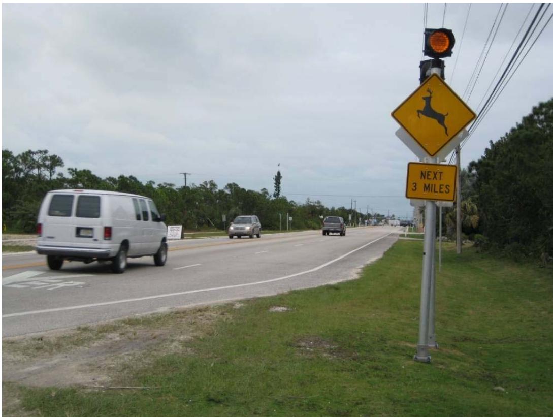
Figure 141. Permanently flashing warning signs for Key deer along U.S. Highway 1 on Big Pine Key (copyright: Marcel Huijser).
