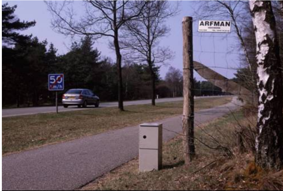
Figure 93. An infrared break-the-beam animal detection system (manufactured by Calonder Energy, Switzerland) at a gap in a wildlife fence near the town 't Harde, The Netherlands (copyright: Marcel Huijser).
