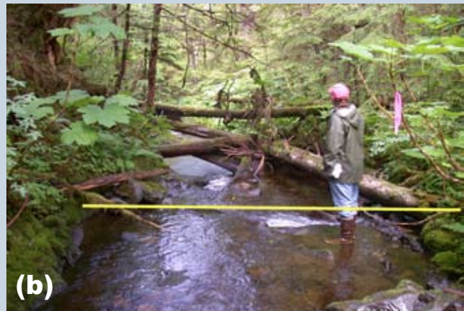
Figure 5.5—(a) Bankfull elevation on an unentrenched alluvial channel. (b) Ordinary high water elevation in an entrenched coarse-grained channel without depositional features.
