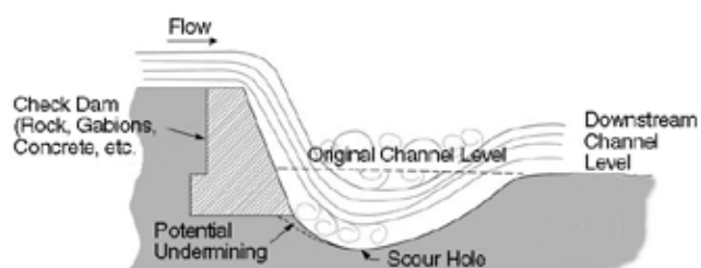
EFFECTS OF WATER SCOUR AT TOE OF A CHECK DAM OR WATERFALL
