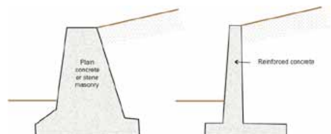
FIGURE 33 Cross section of gravity (left) and cantilever (right) retaining walls (Adapted from Das 2007).
