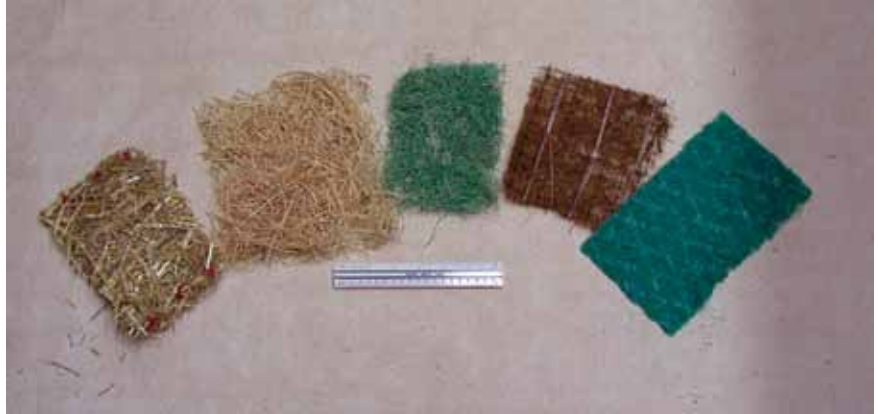
Figure 3-7—Erosion control blankets (l to r) – straw, excelsior (natural), excelsior (dyed green), coir, and netless wood/synthetic.
