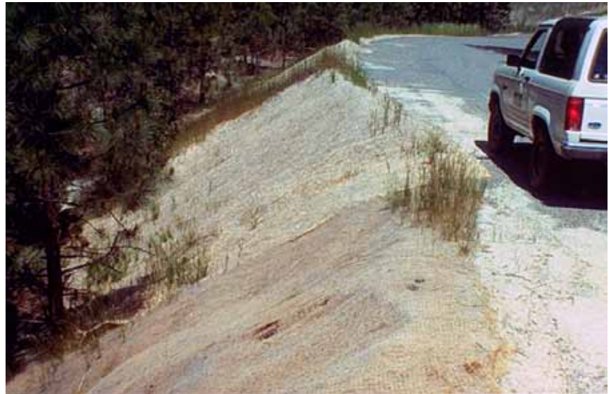
Figure 3-8—Erosion control blankets in a field test section to determine the most cost-effective erosion control material for the fillslope.
