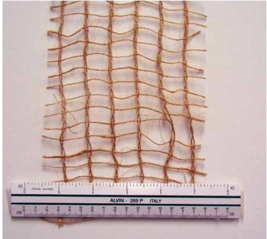
Figure 3-5—Close-up of erosion control net, a natural coir fiber.
