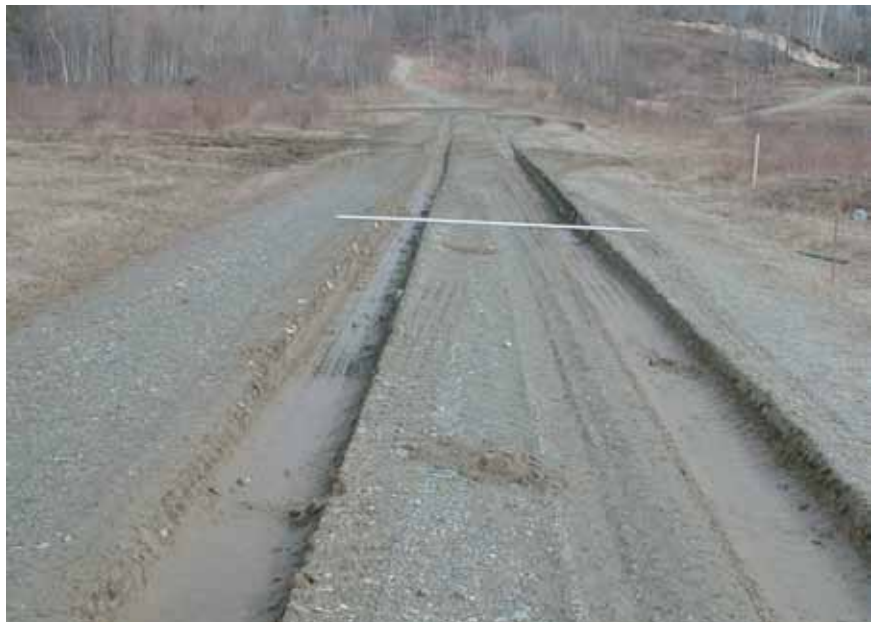
Figure 3-58—Photos showing the advantages of reduced tire pressure to reduce rutting depth (photos from Maureen Kestler).
