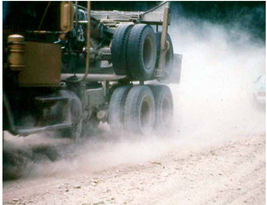
Figure 2-15—Dust from unpaved roads is not only a nuisance but creates a safety hazard by reducing the driver's visibility.
