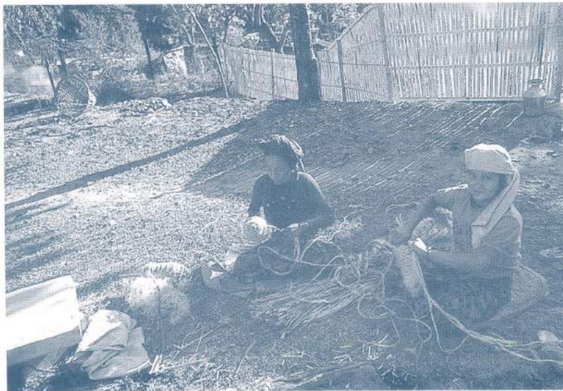
Spinning raw jute into yarn for the production of jute netting
