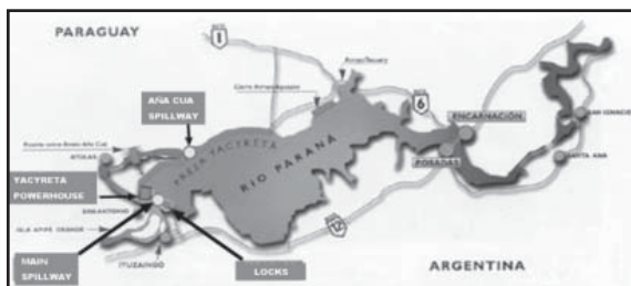
Schematic diagram of the Yacyretá hydroelectric complex showing the location of the spillways, powerhouse, and locks.
