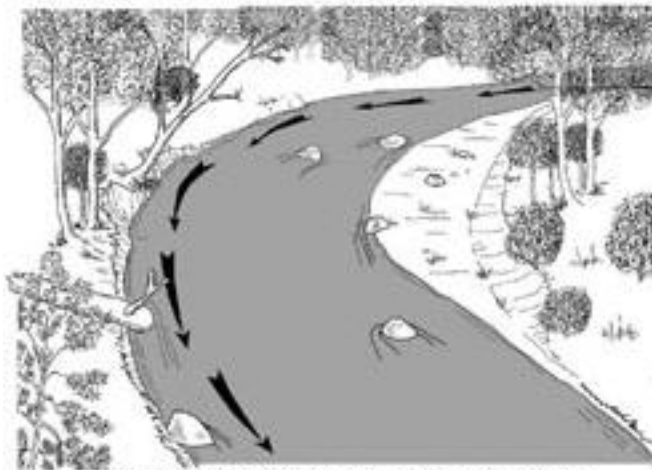
ACTIVE BANK SCOUR WITH VERTICAL CUT BANKS, SLUMP BLOCKS, AND FALLING VEGETATION
